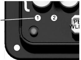
LED ① will apply to the speaker connected to terminals 1 and 2 of the Audio I/O connector (see page 43) and LED ② will apply to the speaker connected to terminals 10 and 11.
