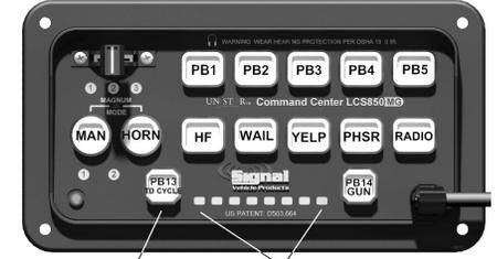
TD CYCLE Button TD Indicator LEDs
