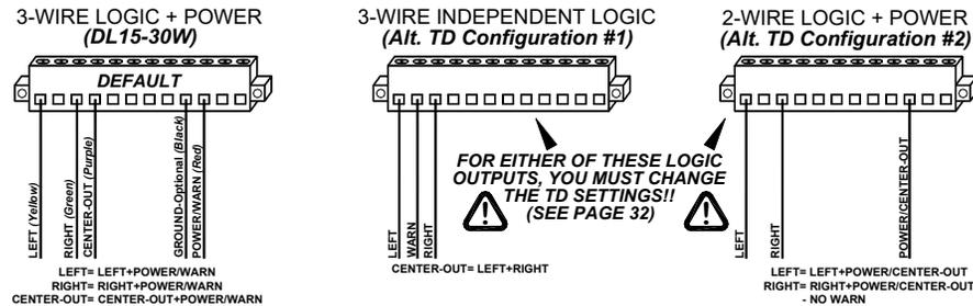
If you will be using the **TD CYCLE** button on the LCS850MG control head to operate your "logic controlled" traffic director i.e. its own internal controller, please verify that DIP switches 3 and 8 on the back of the control head are set properly. (See pages 5 & 7)
