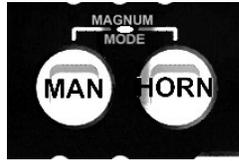
In many modes, the siren's Air Horn can also be activated by pressing the vehicle's horn switch (if you have connected your Horn Ring Transfer to Terminals 7 & 8 of the 12-terminal Audio I/O connector as described on pages 43-44). The chart below summarizes the functionality of the AUX terminal/HRT.
