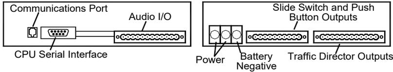
Electrical connections to the unit are made using several terminals and removable connectors located on both the front and back of the unit. The unit is protected by a 20 amp fuse on the input power and each output is protected by a 20 amp fuse. Wiring diagrams on pages 41 and 44 show detail of how to make all of the necessary electrical connections.
