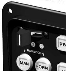
**WARNING!** Once you have programmed all necessary options, **you must flip the Programming Mode DIP switch down to save the changes.**
