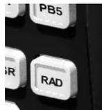
To use the RADIO button to control the **PB13** output, flip DIP switch 11 up.
