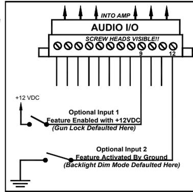
**Please note:** By default the Gun Lock button WILL NOT operate unless you have +12VDC applied to terminal 9 of the AUDIO I/O connector. To bypass this feature, connect Terminal 9 directly to +12VDC or Program as described below (PB14 and MAN Green)
