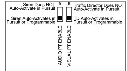
**PROGRESSIVE ENABLE (Progressive Slide Switch Enable)**
