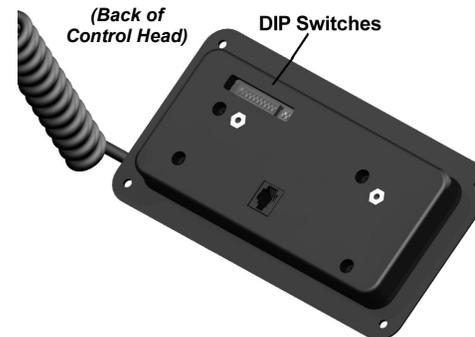
There are 14 DIP switches located on the back of the Control Head. The default position for all of them except for Gun Lock (DIP switch 2) is "down".
