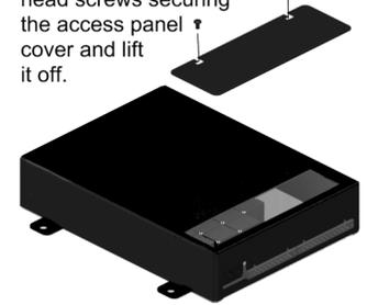
1. To access the fuses, loosen the two Phillips head screws that secure the access cover to the top of the siren, and remove the cover.
