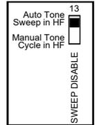
If, when in HF mode, you only want the siren to automatically “sweep” through all of the other tones when the siren is activated by the AUX input/HRT, and you DO NOT want the tones to sweep when the siren is activated by Slide Switch ③, then change this setting:
