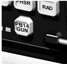
Button is **Green**: (Default setting for **PB1-PB5, PB13**) Button operates as a standard ON/OFF pushbutton switch.
