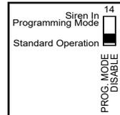
After programming the siren, return the switch to the Standard Operation location to "SAVE" the programming.
