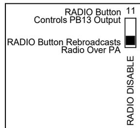
**PHASER ENABLE (Optional Phaser Tone or ON/OFF Switch for the PB13 output)**
