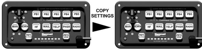
1. After programming the first LCS850MG-CH (control head), make sure it is connected to the amp (this will be the Master Amp), turn it on by applying power to the one of the Power wires and the Remote Enable wire (terminal #4 of the 12-way connector). The Ground wire should also be connected. Ensure slide switch is in the OFF position.
