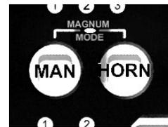
Normally, the siren will automatically be in Magnum Mode when a siren tone is activated. See the **Magnum Mode** DIP switch section on page 7 if you DO NOT want the siren to automatically be in Magnum Mode when a tone is activated.
