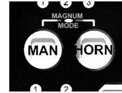
**Manual (MAN):** In Standby (no Audio Modes activated) or Hands Free Mode, this momentary push button switch provides a manually activated “**Momentary Wind Up**” siren tone while being pressed.
