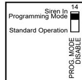
Flip DIP switch 14 up, placing the unit into Programming Mode.
