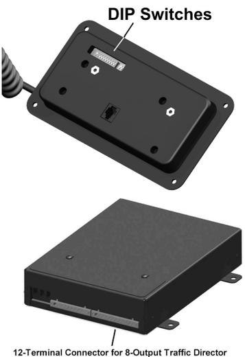
Review the appropriate diagram above and connect the necessary wires from your traffic director harness to the corresponding terminals on the 12-terminal connector that plugs into the back of the LCS850MG-AMP box.
