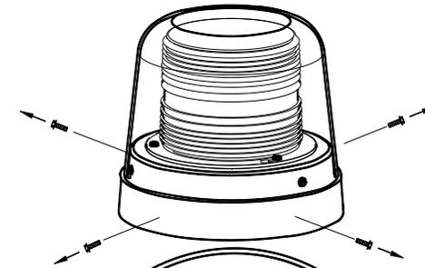
1. Remove the four screws in the side of the aluminum housing.
