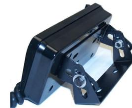
The standard control head can be mounted using the adjustable "U" bracket provided, or directly mounted to a plate or other flat surface. Select a location such as the dash, the overhead console, or a center console. Choose a mounting location convenient to the operator and away from any air bag deployment areas. Consider wire routing and access to connections when selecting location.
