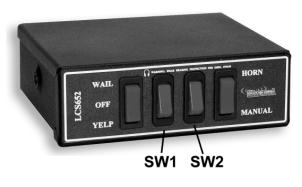
**Please Note:** The two red wires on pins 4 & 8 (LCS652 only) supply the power for the devices switched by SW1 and SW2. Connect the red wires from Pins 4 & 8 through an appropriate user supplied fuse (up to 20 amps). It is **highly recommended** that you appropriately fuse these input wires. Damage to the siren caused by shorts in the devices connected to SW1 or SW2 will not be covered under warranty.
