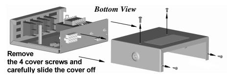
Once the cover is removed, you may move the necessary jumpers over from the "Extra" slots.
