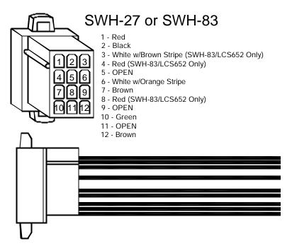
You should make all electrical connections to the wiring harness before installing the connector on the amplifier. If the amplifier ever needs service, the connector can be easily removed from the amp without unwiring it.
