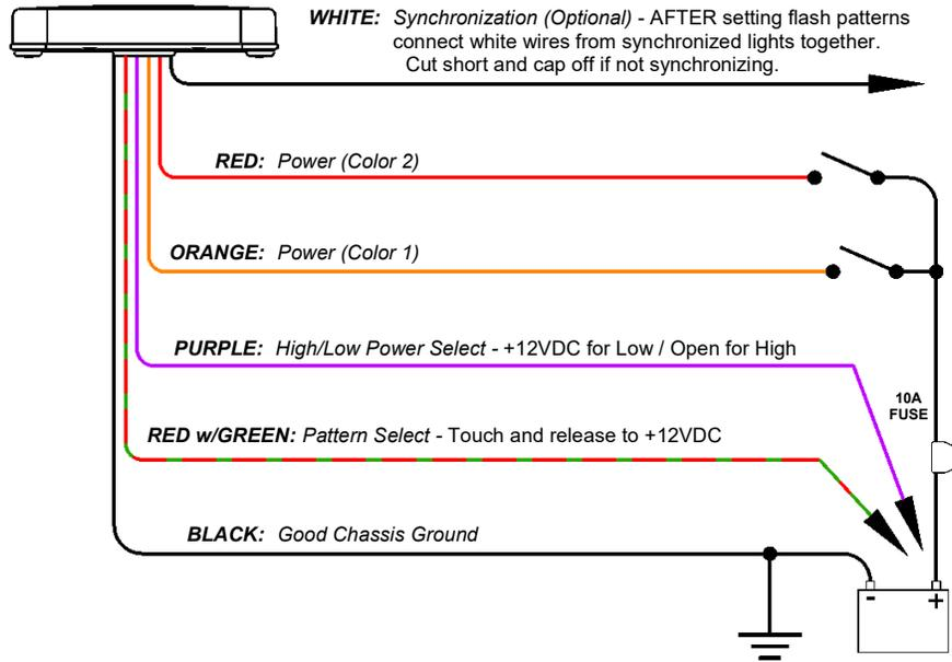
**White** - (Synchronization) Used to synchronize two lights together. If you are only installing one unit, cut the White wire short and tape the end. If you will be synchronizing two or more approved synchronizable lights, leave the white wire disconnected for now. Connect the white wires from both units together **ONLY AFTER PROGRAMMING** them for the same **Pattern Type** (see Pattern Programming).
