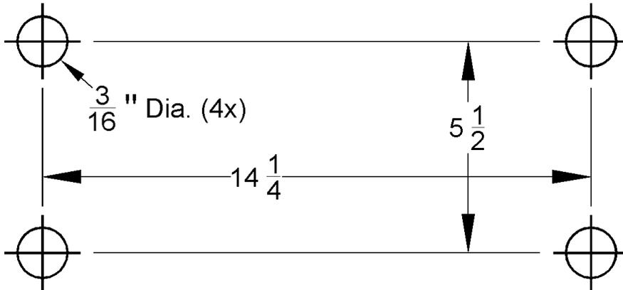
4. Check the underside of the marked locations to ensure that you do not damage any wires or other components. Drill a 3/16" hole in the four marked spots for the mounting bolts, and one in the center for your wires (if applicable). **CAUTION: Take care not to drill through the headliner below.**
